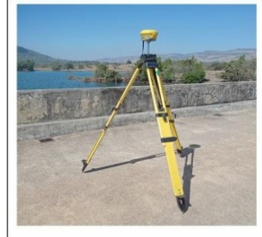
Base Station Setup on Dam Top
