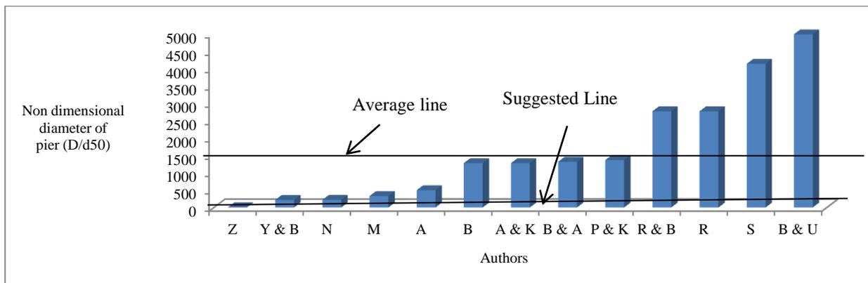
Figure 6: Variation in non-dimensional diameter of bridge pier w.r.t d<sub>50</sub> (D/d<sub>50</sub>)
