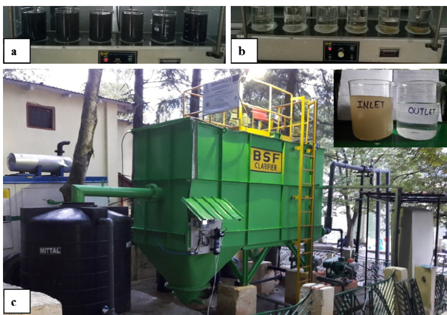
Fig. 5: Pictorial view of Jar apparatus with (a) Raw water (b) Settled water (c) Pilot Plant installed at Nainital
