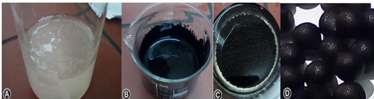
Fig. 1: Preparation of alginate beads with entrapped activated carbon (AG-AC).
