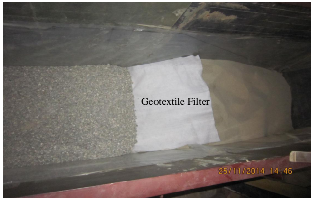
Fig. 7: Model Test Showing Geotextile Filter, As A Replacement To Conventional Granular Filter
