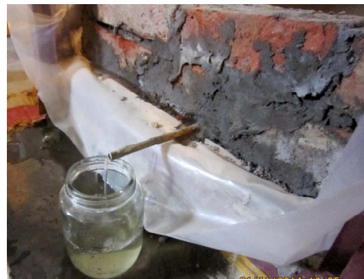
Fig. 3: Collecting the Water Seeped Through Earthen Dam Cross- Section
