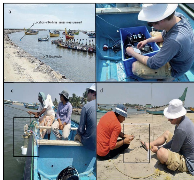
Fig. 2. (a) Location of temporal measurement of radon concentration; (b) and (c) RAD7 and RAD-Aqua water exchanger system for the spatial survey of radon concentration in seawater using boat; (d) Pore-water sample collection
