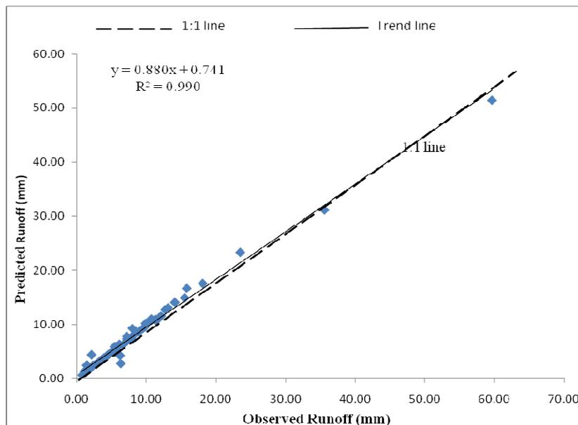
**Fig. 10: Comparison between observed and predicted daily runoff without extreme rainfall events for model validation.**
