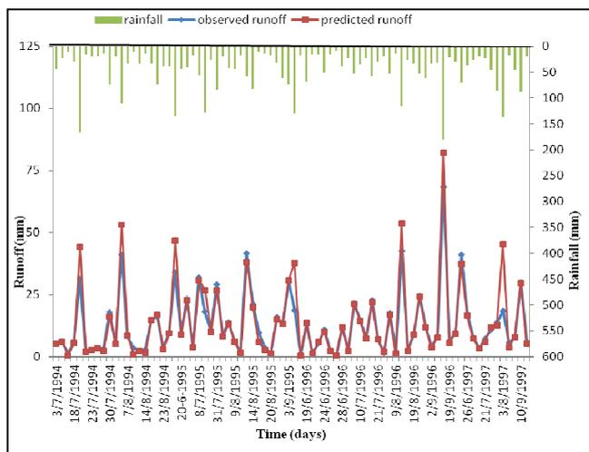
**Fig. 6: Observed and predicted daily runoff hydrographs for model calibration period (1994-1997)**
