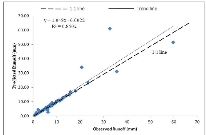
**Fig. 9: Comparison between observed and predicted daily runoff for model validation.**
