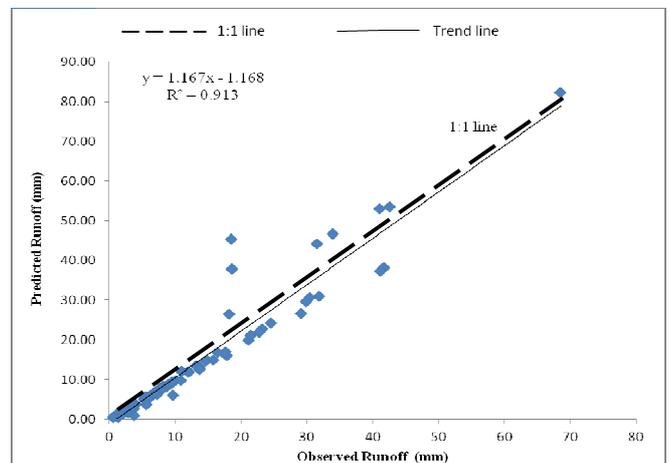
**Fig. 7: Comparison between observed and predicted daily runoff for model calibration.**
