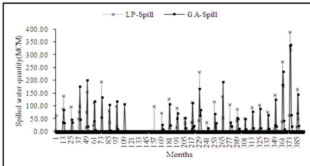
**Fig.9. Spilled water quantity by LP and GA methods**
