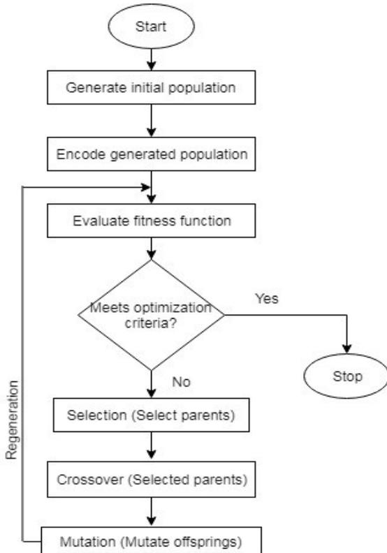
**Fig.5. Flowchart of a typical GA model**
