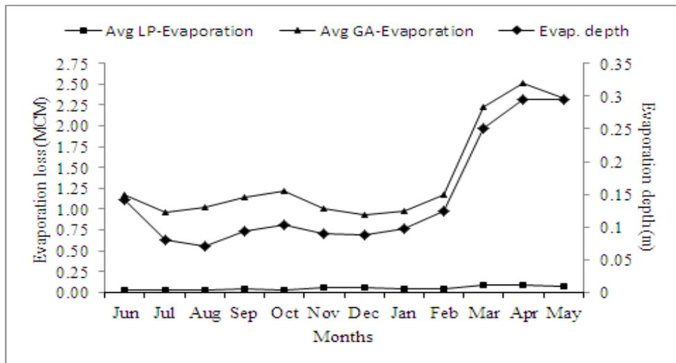
**Fig.8. Average monthly evaporation depth and losses**
