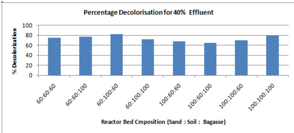
**Fig. 4: Percentage Decolorization in Batch 2 reactors**
