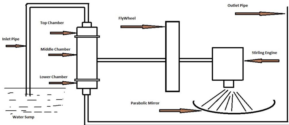
**Fig. 7: Solar powered stirling engine based water pumps (Saini, Kohli et al.)**
