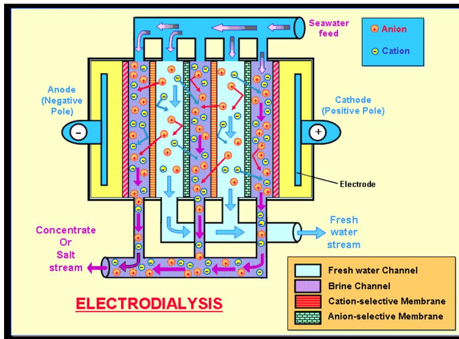
**Fig. 9: The electro-dialysis desalination technology (Tautai Foundation 2015).**
