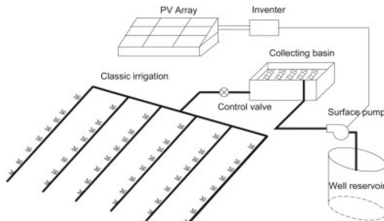
**Fig. 2: Schematic layout of photovoltaic irrigation system (Gopal, Mohanraj et al. 2013).**
