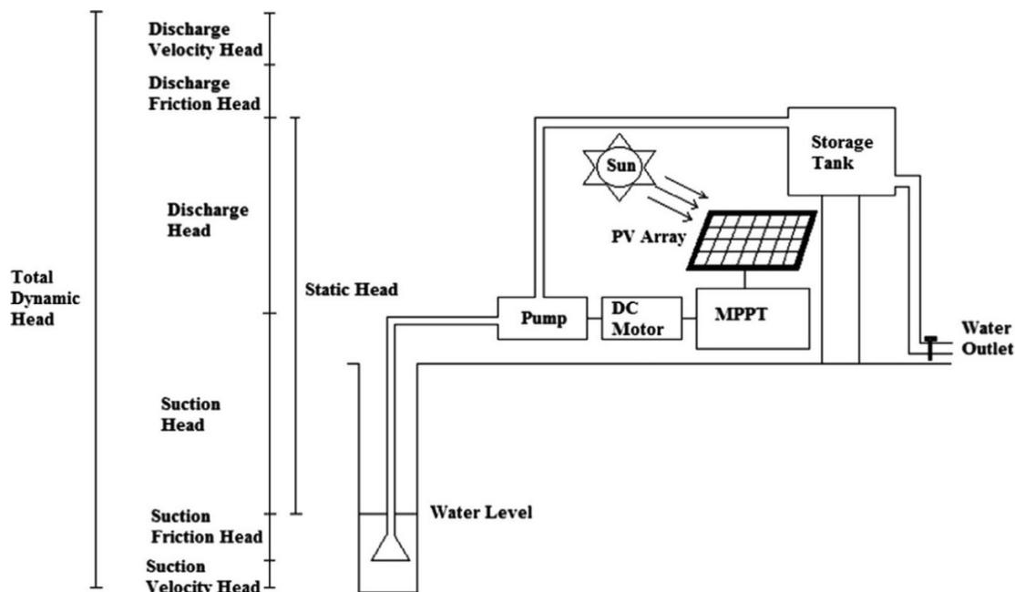
**Fig. 1: Schematic of a direct coupled solar photovoltaic water pumping system with MPPT (Chandel, Naik et al. 2015).**
