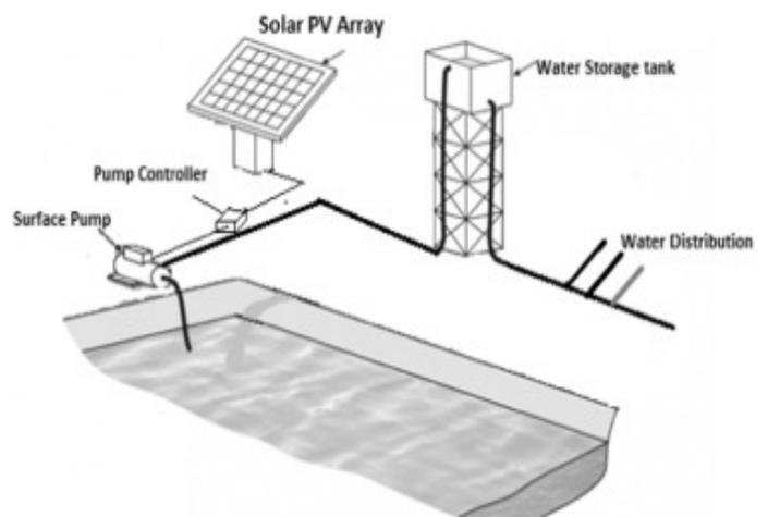
**(a) Using surface mounted pump**
