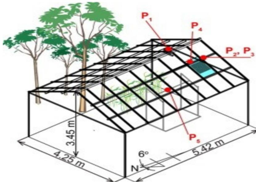
**Fig. 5: Semi-transparent PV based greenhouse (Cossu, Yano et al. 2016).**
