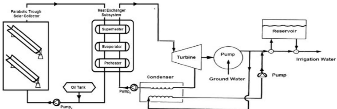
**Fig. 6: Parabolic trough collector based STEWP (Bataneh 2016).**
