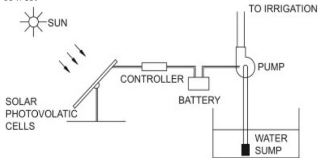
**(a) Using surface mounted pump**
