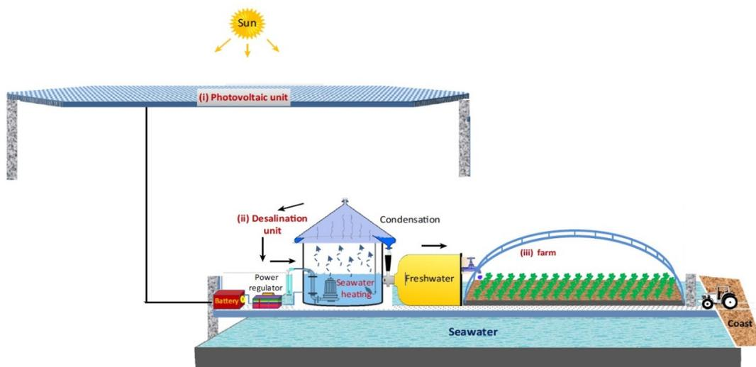
**Fig. 8: Schematic of solar powered desalination system for irrigation (Moustafa 2016).**
